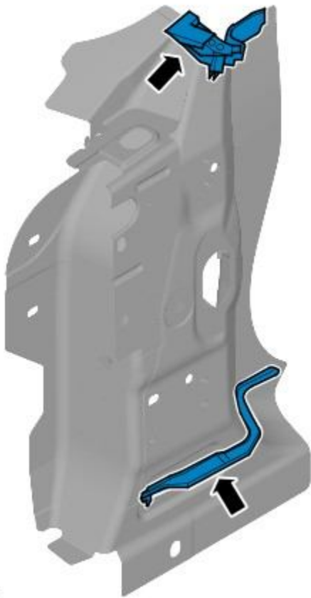
Expanding Foam Acoustic Seals - A-pillar, (upper)
