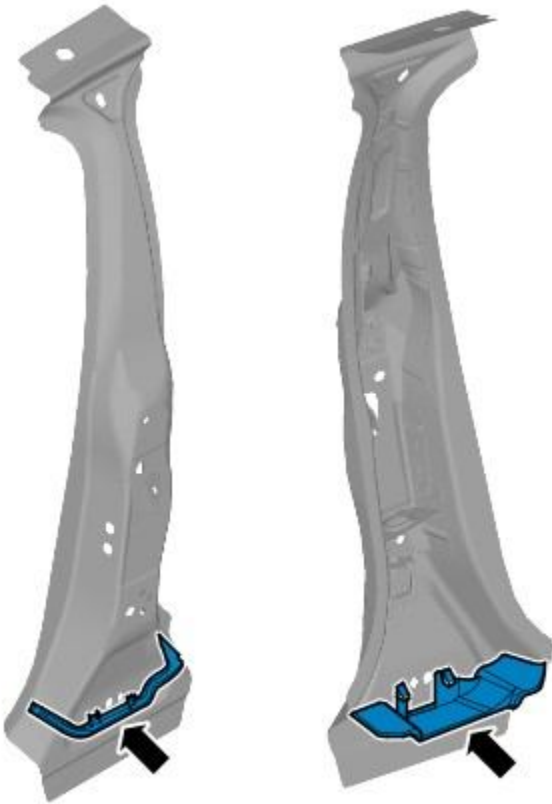
Expanding Foam Acoustic Seals - B-pillar, (reinforcement)
