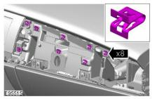
6. Install the clips into the instrument panel.
