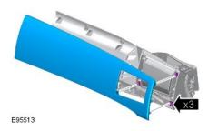
8. NOTE: When removing the component, some of the clips may remain attached. These clips should be removed and returned to their original positions in the passenger side register carrier.
