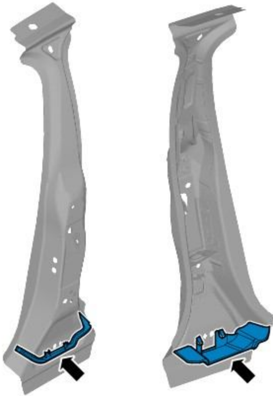
Expanding Foam Acoustic Seals - B-pillar, (reinforcement)
