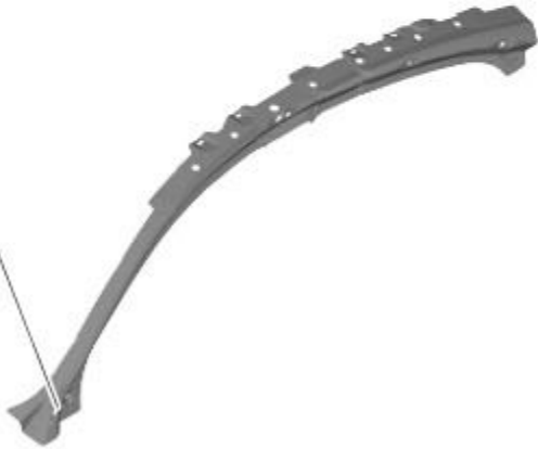
Expanding Foam Acoustic Seals - B-pillar, (reinforcement)
